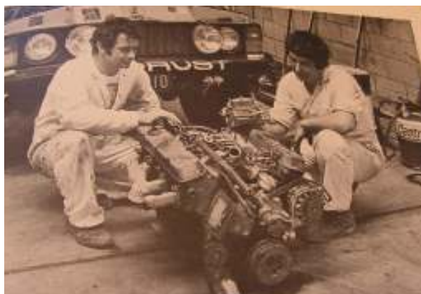
P76 V8 for Range Rover preparation
